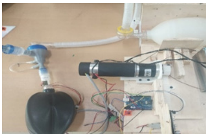
Figure 2: Setup showing compression of a bag valve mask using DC servo motor with an encoder.
