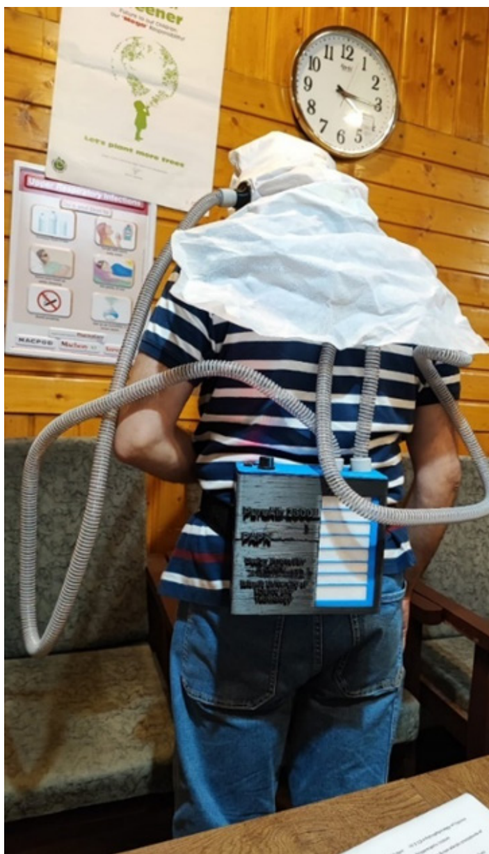
Figure 13: Headgear Unit Connected with Air handling Unit Via 2Nos. BiPAP Pipes
